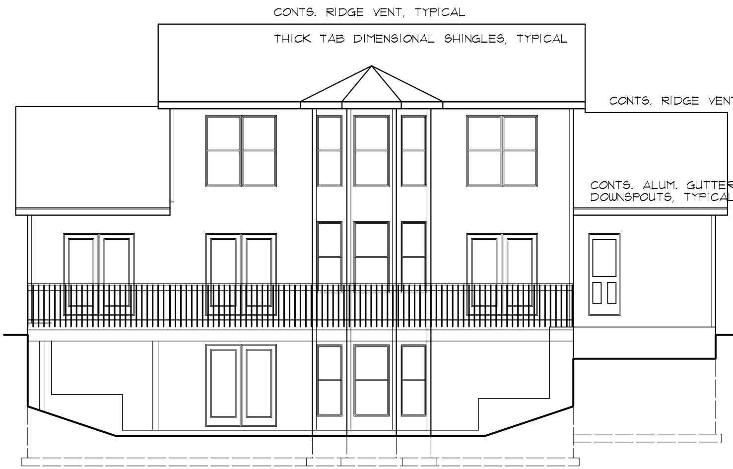
REAR ELEVATION SCALE: 1/8"=1'-0" ON 11X17 1/4"=1'-0" ON 24X36
